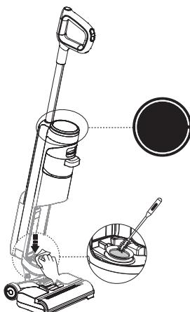
When LED loop illuminates red, remove Dirty Water Tank, clean the dirt sensor with a damp cloth or cleaning tool.
