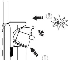
Place the tank back into the appliance. You should hear a "Click" if done correctly.
