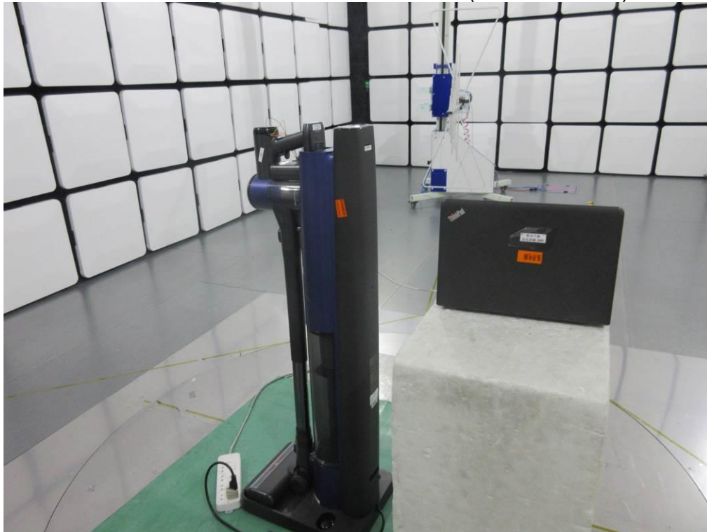
RADIATED RF MEASUREMENT SETUP (30MHz ~ 1 GHz)
