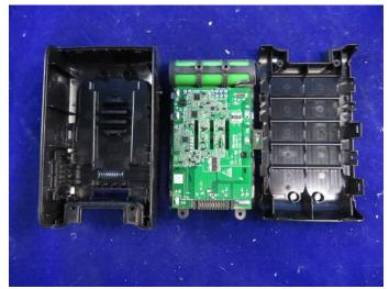
internal view of battery pack VS15-02
