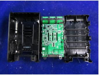
internal view of battery pack VS15-01
