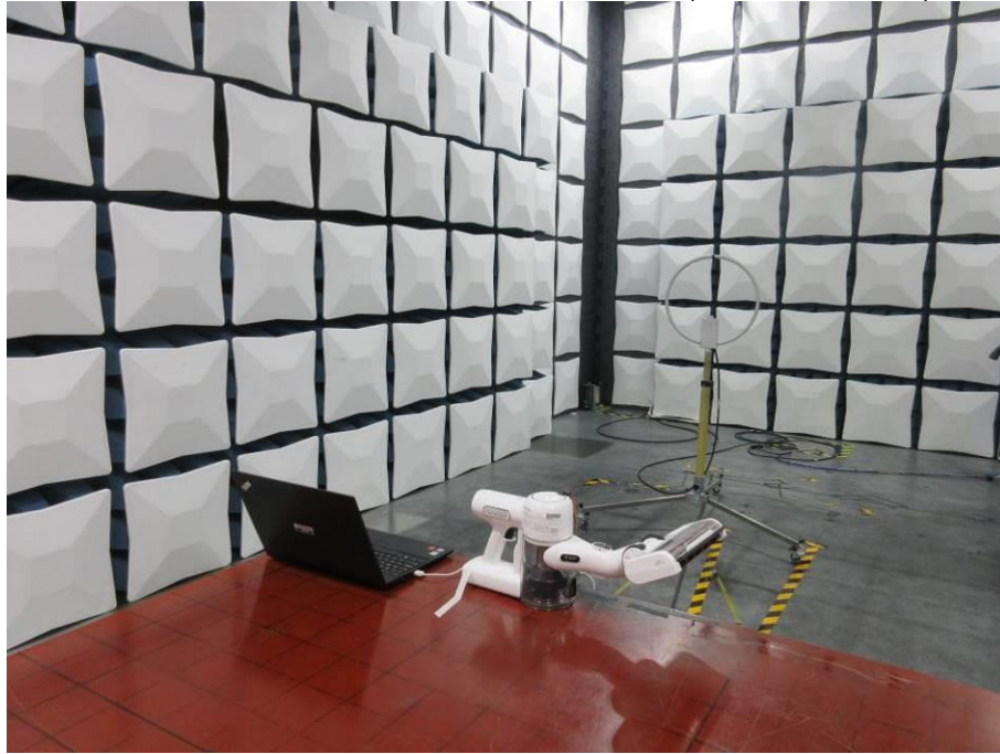
RADIATED RF MEASUREMENT SETUP (9KHz ~ 30 MHz)
