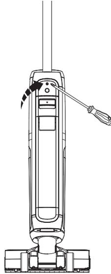
In the event that the handle needs to be disassembled, press the spring to release the handle with a tool (like a screwdriver) and lift the released handle from the appliance.
