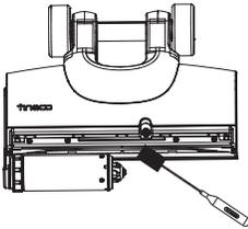
Remove hair and debris from the brush roller chamber and the opening with the cleaning tool.
