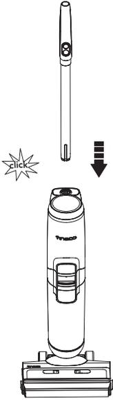
To assemble the handle, insert it into the appliance until you hear a click.
