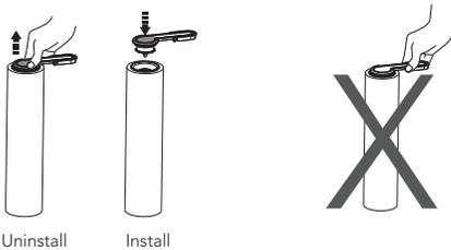
Pull up the roller handle to remove it. Once removed, install the handle into the new brush roller.
