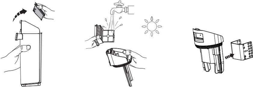
Grasp recessed area on each side of the dry filter and pull upward. Rinse under running water and must be completely dry before recombining with the lid of the DWT.
