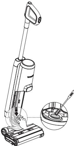
Clean the dirt sensor with a damp cloth or the cleaning tool.
