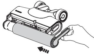
Replace the brush roller by inserting its end into the left side of the holder, then attach the roller tab to the magnetic buckle on the right side to lock into place.
