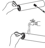
Use the cleaning tool to remove the hair and debris wrapped around the roller and then rinse the roller with water. Replace the brush roller back into the accessory holder, and allow it to dry completely before reinstalling.
