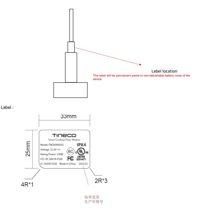
Note: 1. The label will be permanent paste to non-detcahable battery cover of the device. 2. This would be a plastic label with a permanent adhesive.
