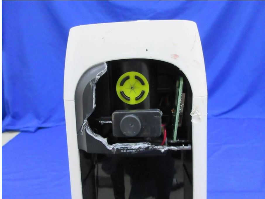
View of RF Module and Antenna location-3
