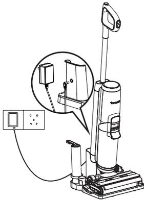
To charge the appliance, place the appliance on the charging base and plug the adaptor into a power outlet.
