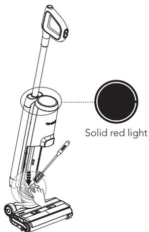
When LED loop illuminates red, remove Dirty Water Tank, clean the dirt sensor with a damp cloth or the cleaning tool.
