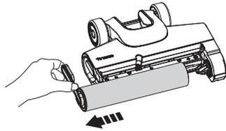
Remove the brush roller by grabbing the brush roller tab and pulling out.
