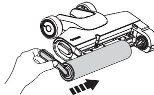
Replace the brush roller by inserting the brush roller end into the right side of the holder, then attach the roller tab to the magnetic buckle on the left side to lock into place.
