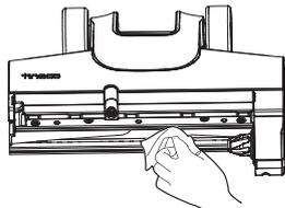
Remove hair and debris from the brush roller chamber and the opening with a tissue or a damp cloth.
