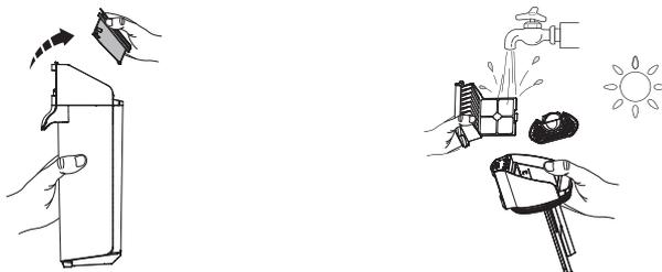
Grasp recessed area on each side of the dry filter and pull upward. Rinse under running water and must be completely dry before recombining with the lid of the DWT.
