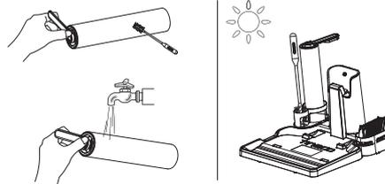
Using the cleaning tool, remove the hair and debris wrapped around the roller and rinse with water. Replace the brush roller back into the accessory holder, and allow it to dry completely before reinstalling.
