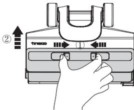
Squeeze latches on the cover and pull upward to remove.
