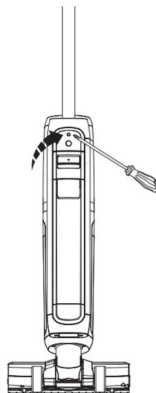
In the event that the product must be returned, please disassemble the handle. Press the spring to release the handle with a tool (like a screwdriver) and lift the released handle from the appliance.
