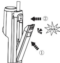
Place the tank back into the appliance. You should hear a "Click" if done correctly.
