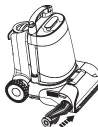
Place the brush roller back by inserting the brush roller end into the right side of the holder, then attach the roller tab to the left side to lock into place.
