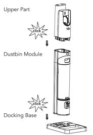
Insert dustbin module into docking base first, then insert upper part into dustbin module.
