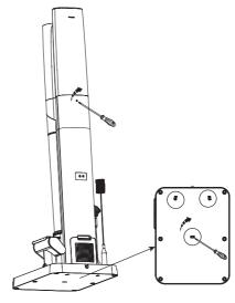
In the event that the Clean Station need to be disassembled, press the latch with tool to remove the three parts.
