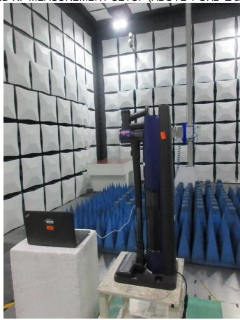
RADIATED RF MEASUREMENT SETUP (ABOVE 1 GHz- Z axis)-Part 2
