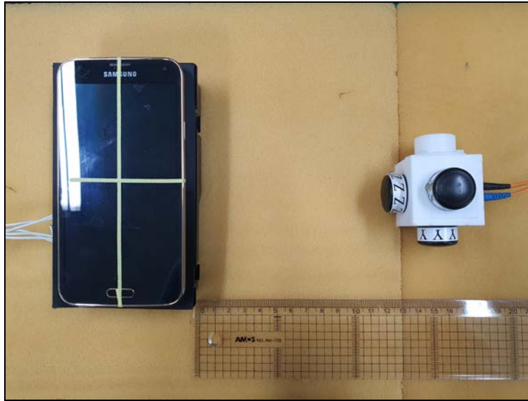
Photo of MPE Test Set up at 10 cm distance (E-field)
