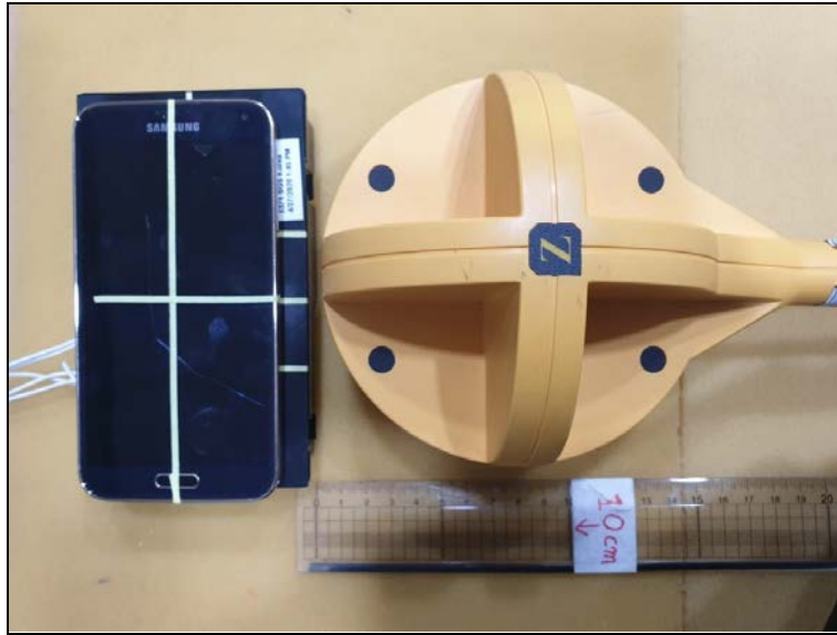
Photo of MPE Test Set up at 6 cm distance (H-field)
