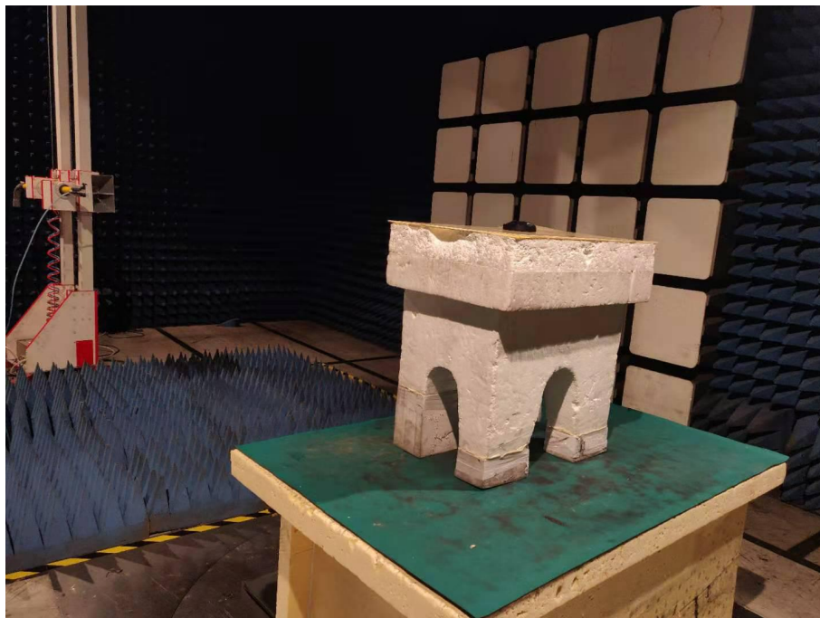
Spurious Emission Test Setup (Above 1GHz)
