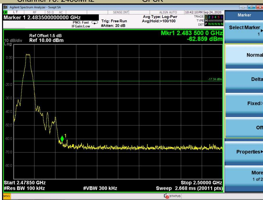
Test Model Maximum Conducted Level RBW=100kHz
