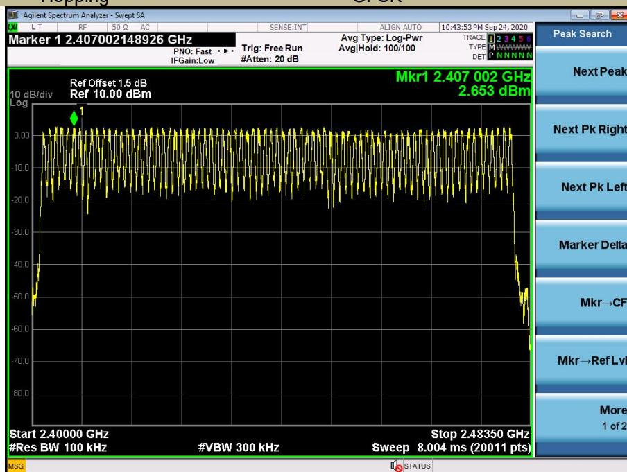
Test Model Conducted Spurious RF Conducted Emission
