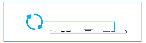
Reset Device by pressing the reset button with a small object, such as a paperclip.
