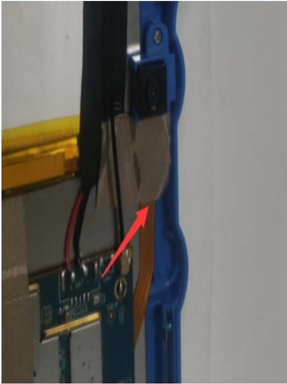
Camera cable is shielded by conductive cloth
