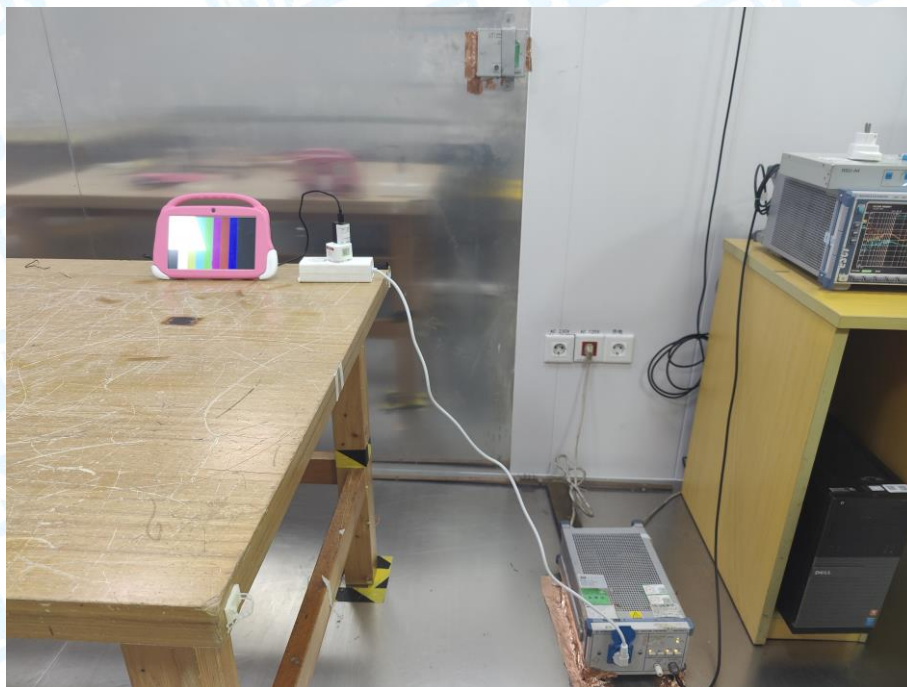
Photo of Setup for Conducted Emission
