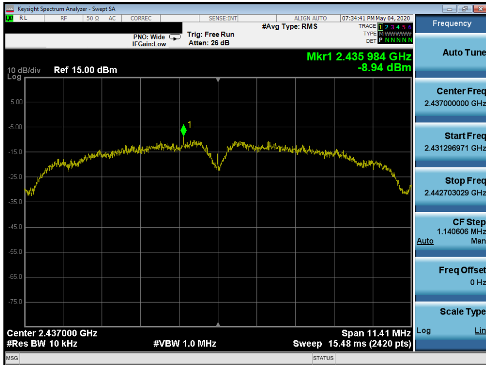
Plot 7-29. Power Spectral Density Plot (802.11b – Ch. 6)
