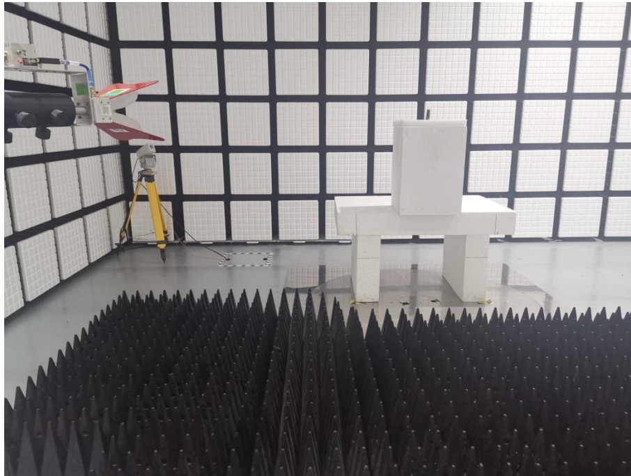
Description: Radiated Emission Test Setup (1 GHz -18GHz)
