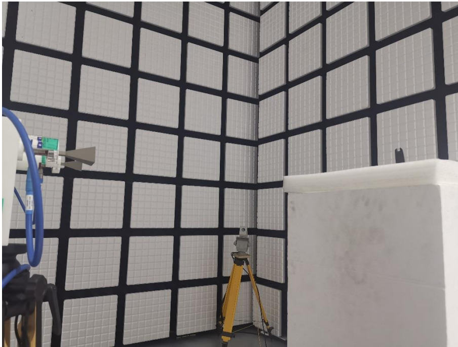
Description: Radiated Emission Test Setup (Above 18GHz)
