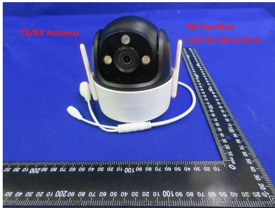
View of antenna
