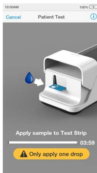
When the sample is detected the Instrument will sound and a confirmation message will be displayed.
