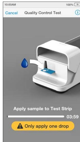
When the Quality Control sample is detected the Instrument will sound and a confirmation message will be displayed.
