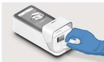
Cleaning the area around the Test Strip slot
