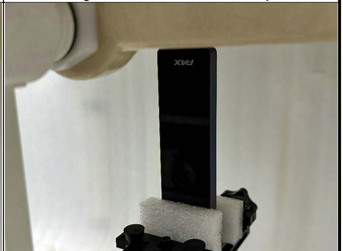
Bottom Side of EUT with 0 cm Gap
