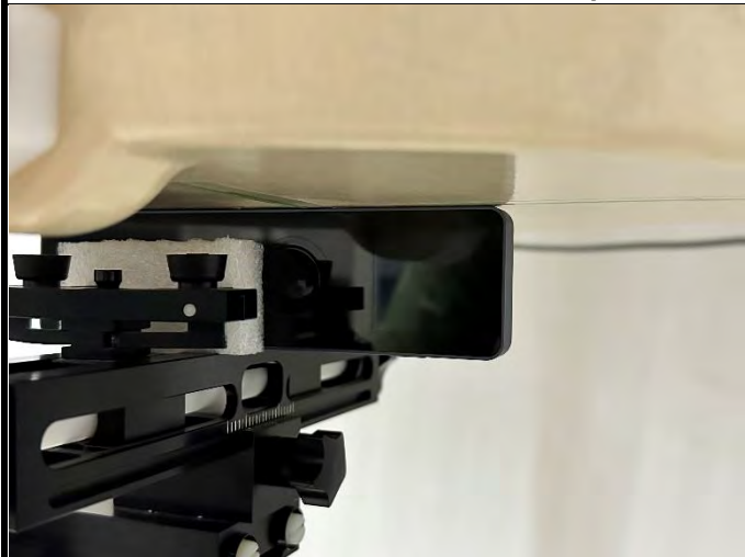
Left Side of EUT with 0 cm Gap
