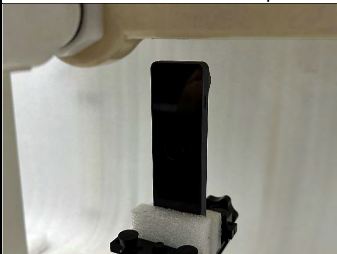
Top Side of EUT with 1.5 cm Gap
