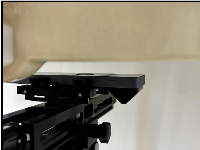
Front Face of EUT with 1.5 cm Gap
