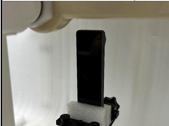
Top Side of EUT with 1.5 cm Gap
