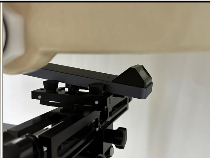
Rear Face of EUT with 1.5 cm Gap
