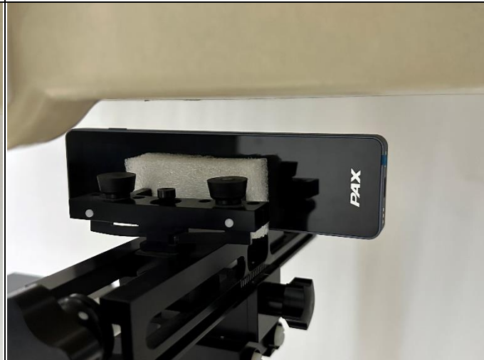
Right Side of EUT with 1.5 cm Gap
