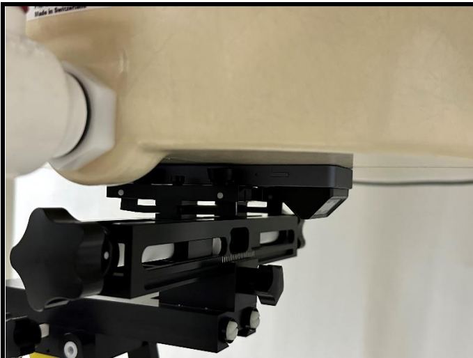
Front Face of EUT with 0 cm Gap
