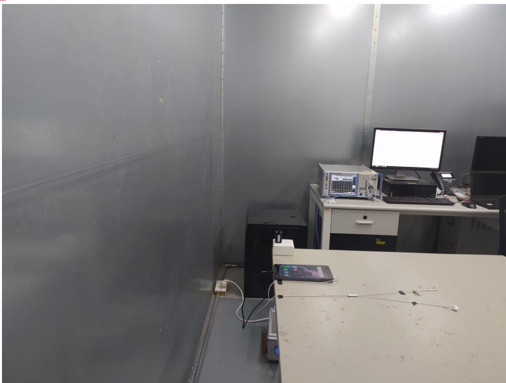
Fig. 3 Power line conducted emission setup photo
