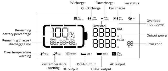
Battery capacity: When power station is being charged, the SOC icon will blink.
