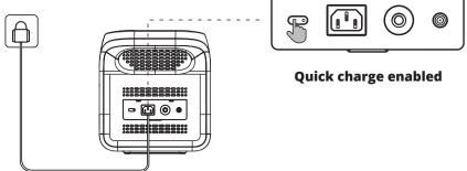
Use standard AC charging cable for fast charging. AC charging cable should plug directly into a 12A (or above) wallmounted socket. We take no responsibilities for any damage caused by using unofficial AC charging cable and other failures to follow instructions.
