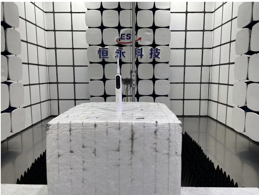
Radiated emission test: Above 1GHz
