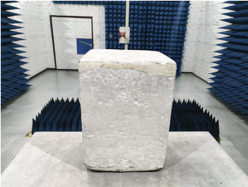
RADIATED EMISSION TEST SETUP ABOVE 1GHz
