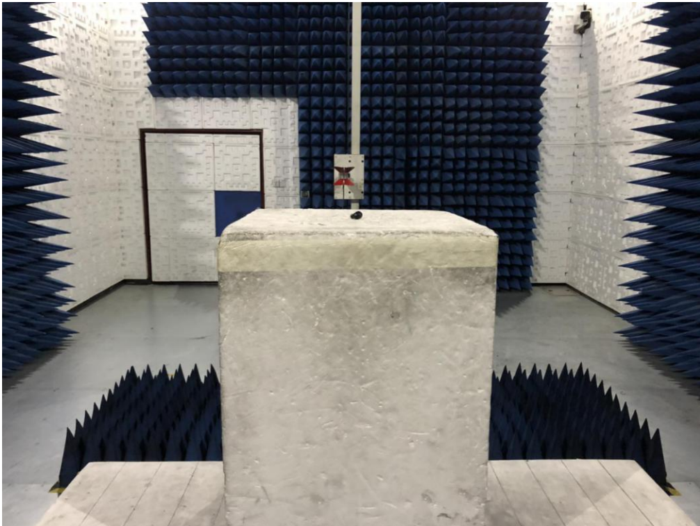
RADIATED EMISSION TEST SETUP ABOVE 1GHZ
