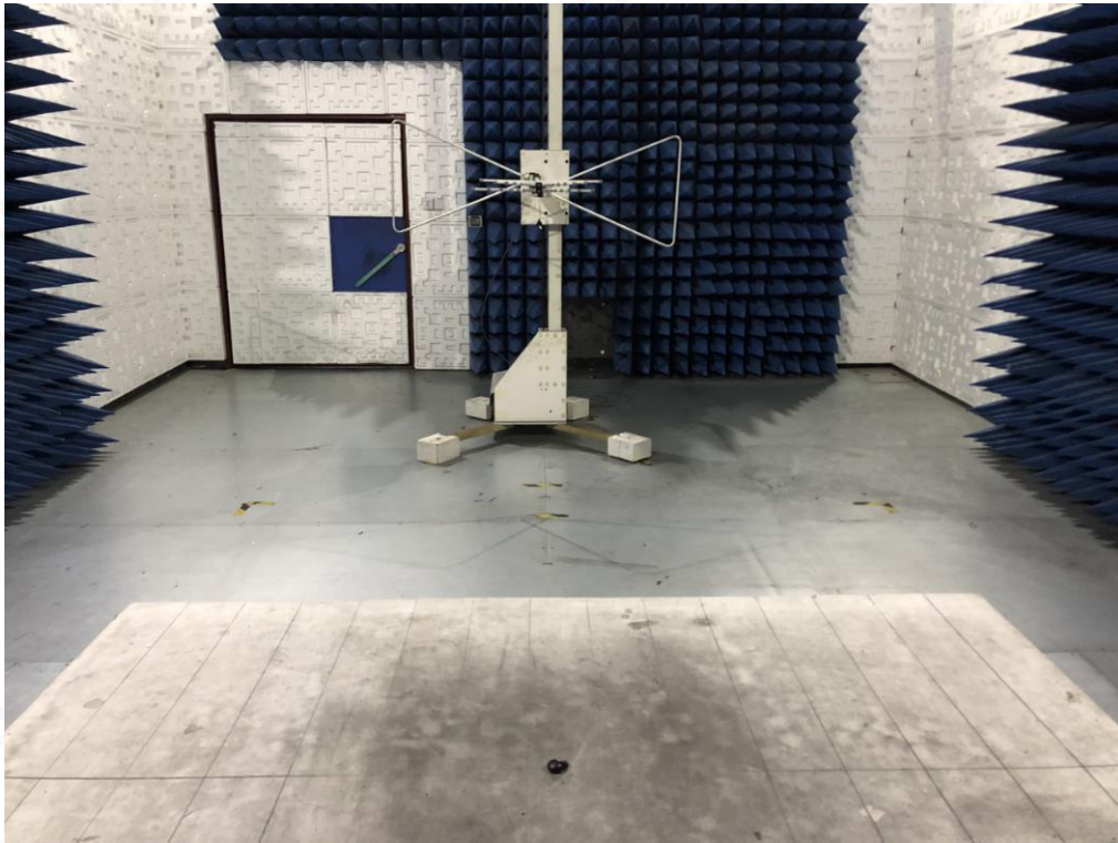
RADIATED EMISSION TEST SETUP ABOVE 1GHZ
