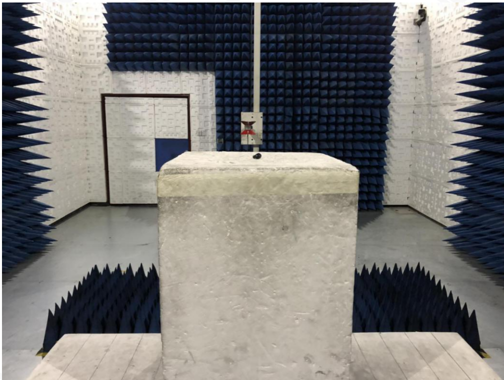
RADIATED EMISSION TEST SETUP ABOVE 1GHZ
