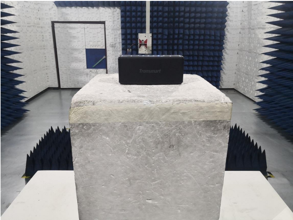
RADIATED EMISSION TEST SETUP ABOVE 1GHz
