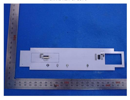
INTERNAL VIEW OF EUT-6(NFC Antenna)
