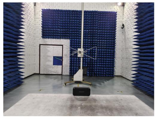
RADIATED EMISSION TEST SETUP ABOVE 1GHz
