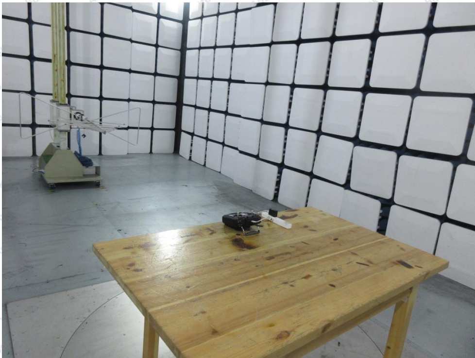
Photo of Radiation Emission Test
