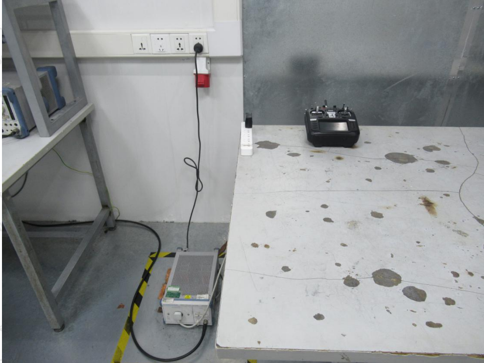
Photo of Conducted Emission Measurement
