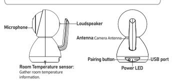
When camera is powered on, press this button and the power LED starts to Pairing button blink, the camera is in pairing mode. Press it again to exit pairing mode
