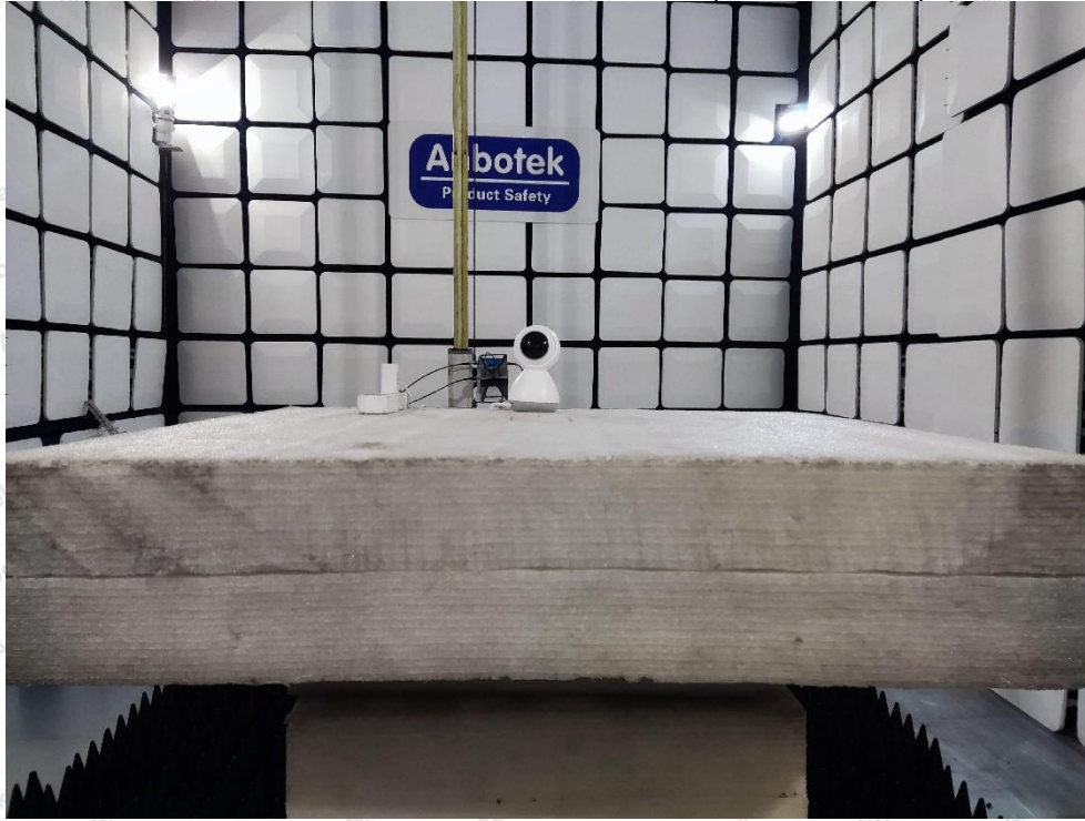
Photo of Radiation Emission Test (above 1GHz)
