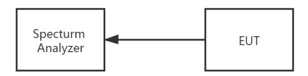
The EUT which is powered by the DC Power, is connected to the Spectrum Analyzer; the RF load attached to the EUT antenna terminal is 50 Ohm; the path loss as the factor is calibrated to correct the reading. Make the measurement with the spectrum analyzer's resolution bandwidth(RBW) = 100 kHz. In order to make an accurate measurement, set the span greater than RBW. **5.4 EUT OPERATION CONDITIONS**
