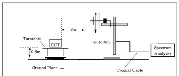
(C) Radiated Emission Test-Up Frequency Above 1GHz
