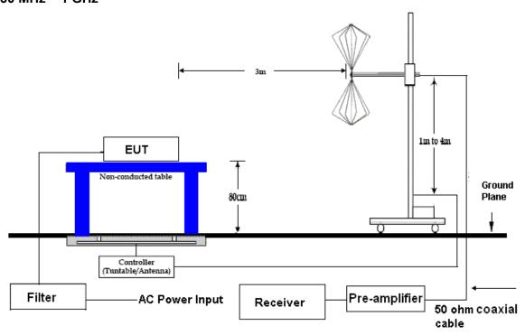
**NOTE:** The EUT system was put on a wooden table with 1.5m heights above a ground plane. For the actual test configuration, please refer to the photos of testing.
