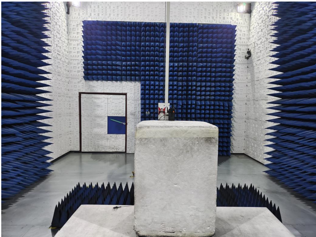
RADIATED EMISSION ABOVE 1G TEST SETUP
