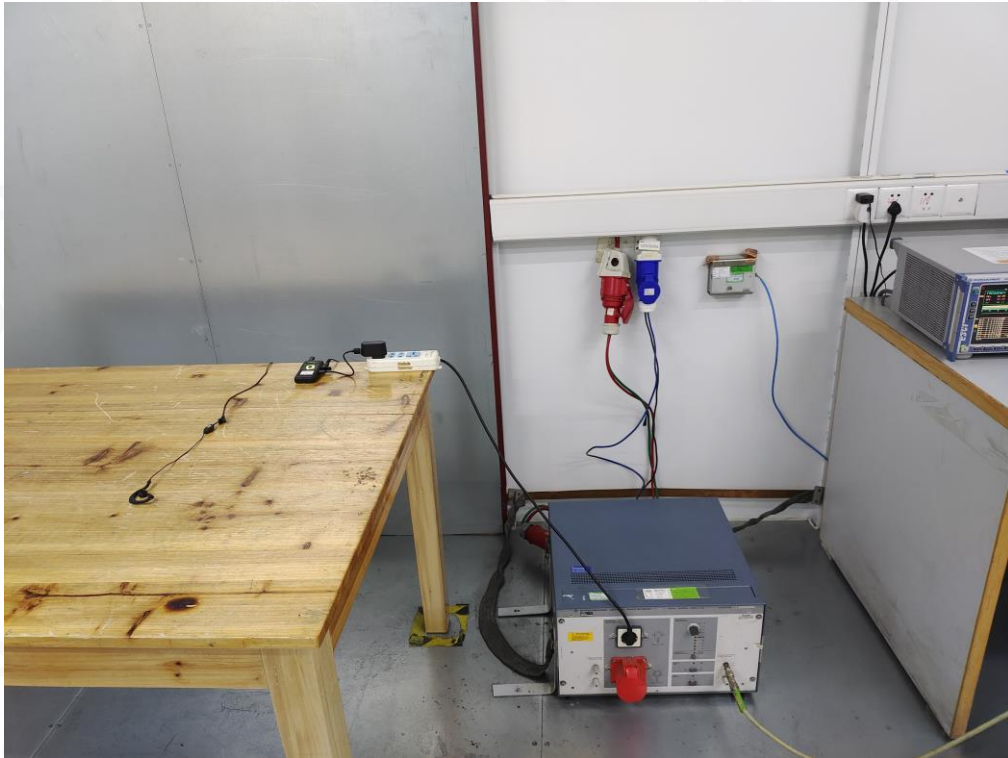
RADIATED EMISSION TEST SETUP-BELOW 1GHZ
