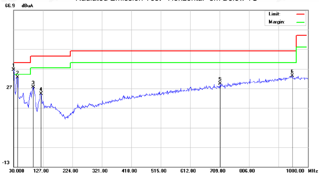
Radiated Emission Test –Horizontal -3m Below 1G
