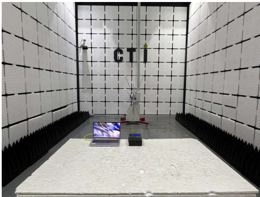
Radiated spurious emission Test Setup-1(Below 1GHz)
