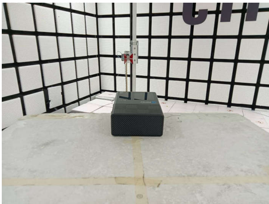
Radiated spurious emission Test Setup-2(Above 1GHz)
