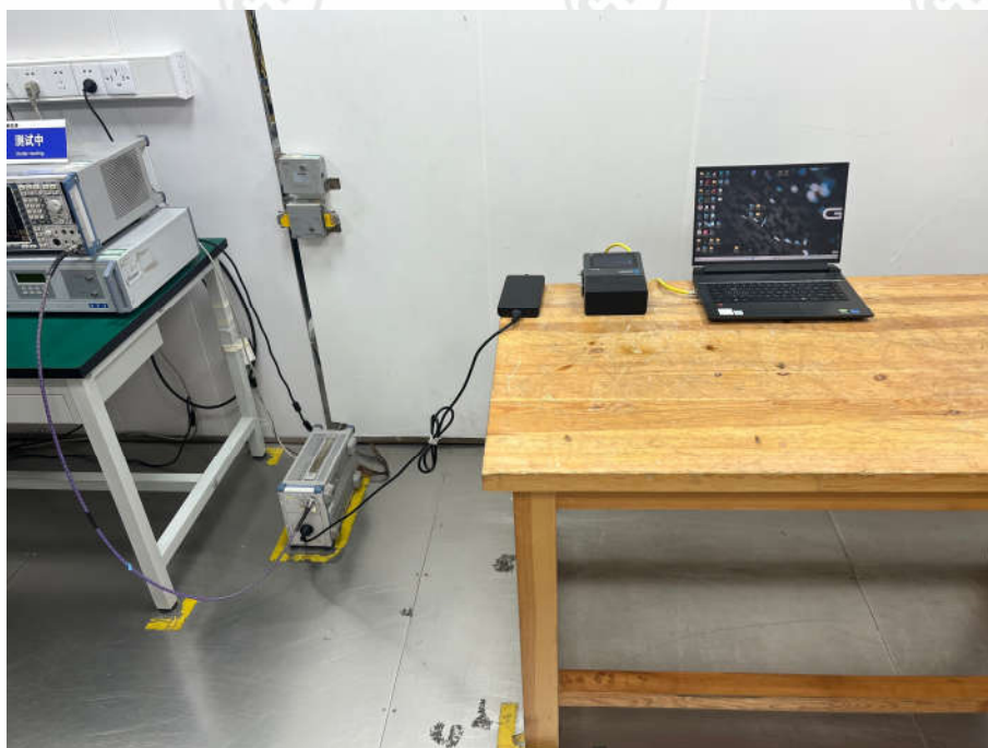
Conducted Emissions Test Setup
