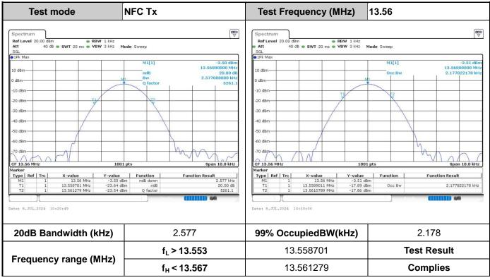
**Remark:** Because the measured signal is CW adjusting the RBW per C63.10 would not be practical since measured bandwidth will always follow the RBW and the result will be approximately twice the RBW.
