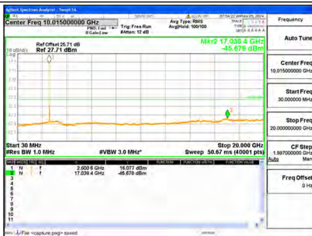
B38-30M-20G / 20MHz / High CH / QPSK
