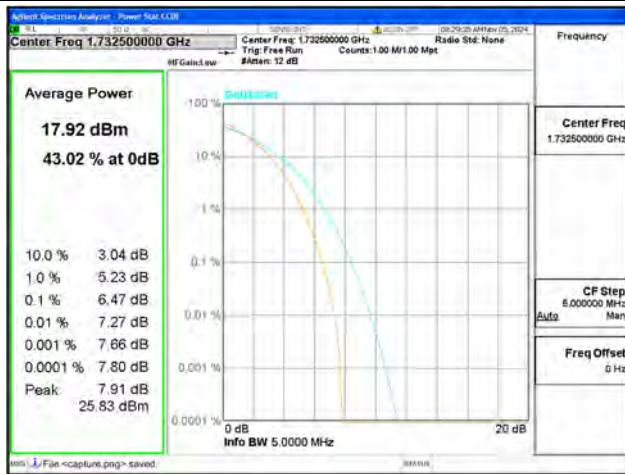
B4 / 3MHz / Mid CH / 64QAM
