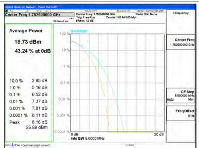
B4 / 5MHz / High CH / 16QAM
