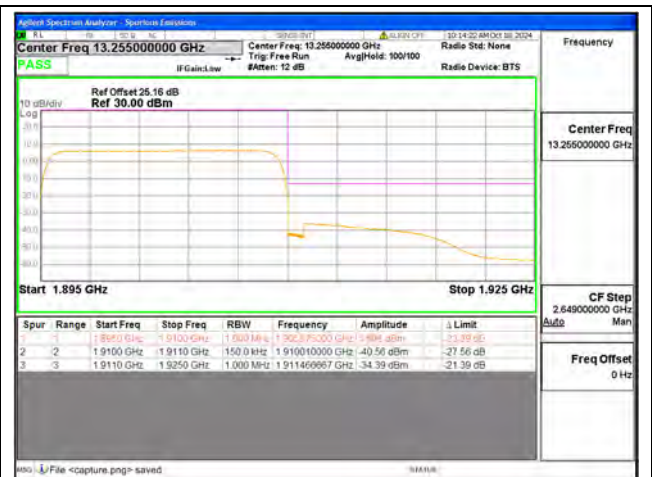
B2 / 15MHz / High CH / QPSK / FULL RB
