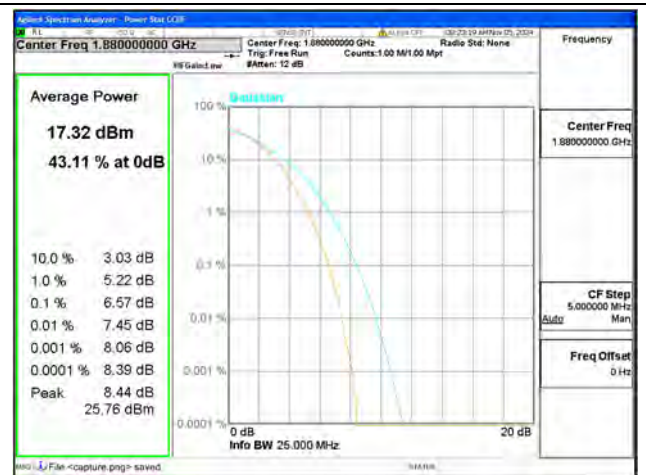
B2 / 15MHz / Mid CH / 64QAM
