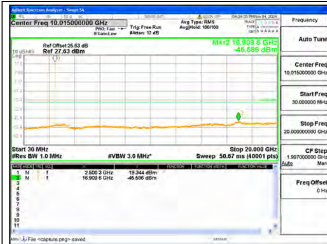
B7-30M-20G / 5MHz / Low CH / QPSK
