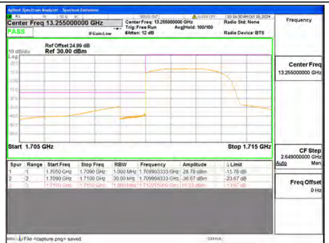
B4 / 3MHz / Low CH / QPSK / FULL RB
