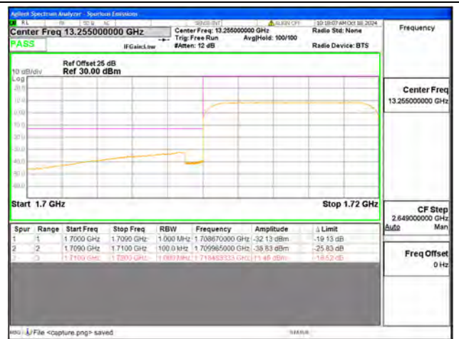
B4 / 10MHz / Low CH / QPSK / FULL RB
