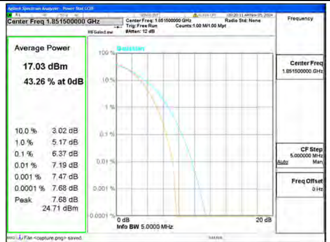
B2 / 3MHz / Low CH / 64QAM
