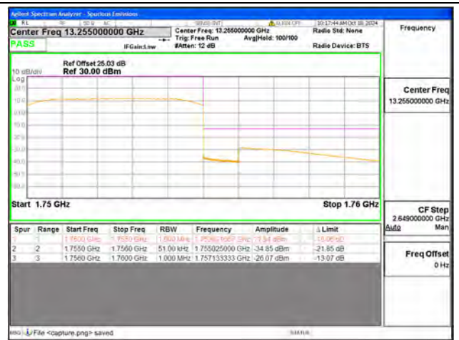
B4 / 5MHz / High CH / QPSK / FULL RB
