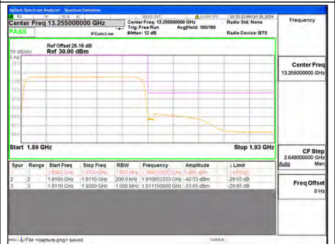
B2 / 20MHz / High CH / QPSK / FULL RB
