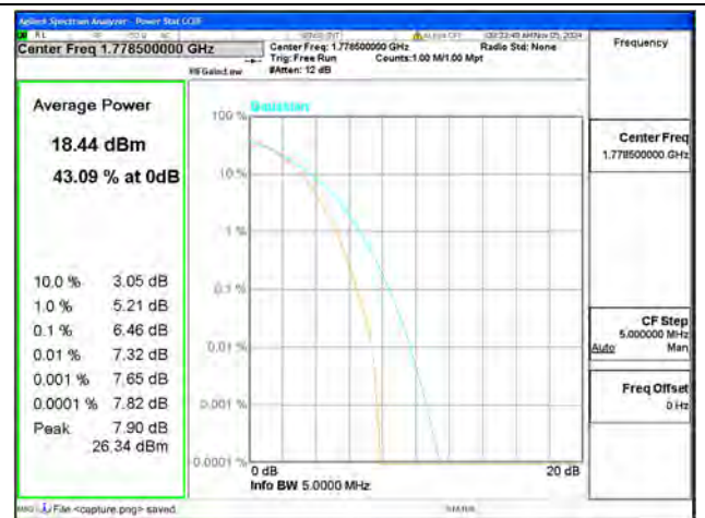
B66 / 3MHz / High CH / 64QAM
