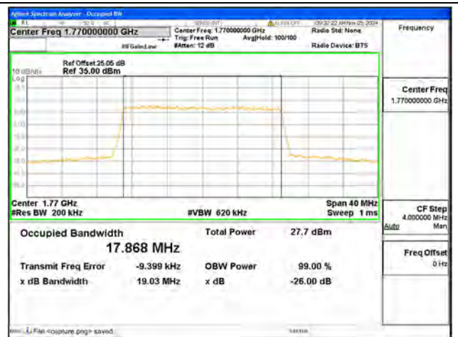
B66 / 20MHz / 64QAM/ High CH
