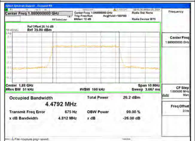
B2 / 5MHz / 64QAM/ Mid CH
