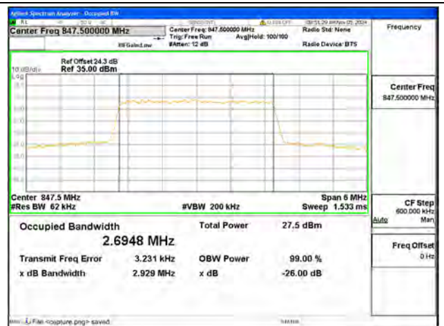
B26 / 3MHz / 64QAM/ High CH
