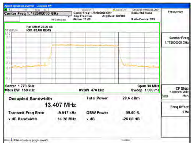
B66 / 15MHz / 16QAM/ High CH
