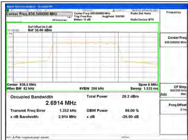
B26 / 3MHz / QPSK/ Mid CH
