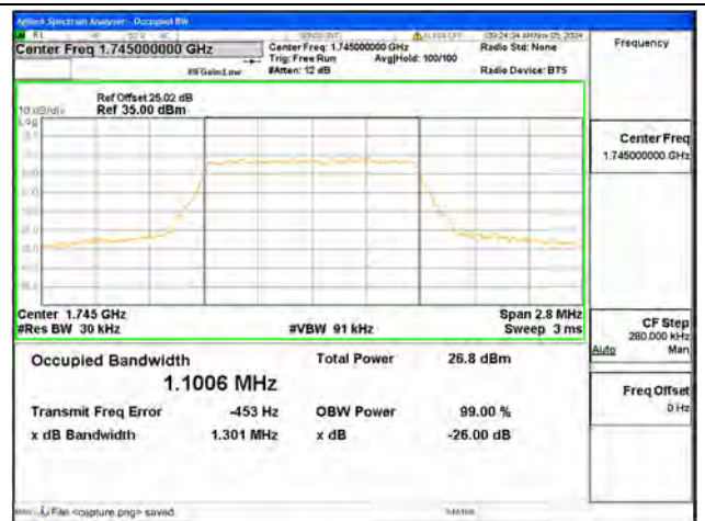
B66 / 1.4MHz / 64QAM/ Mid CH
