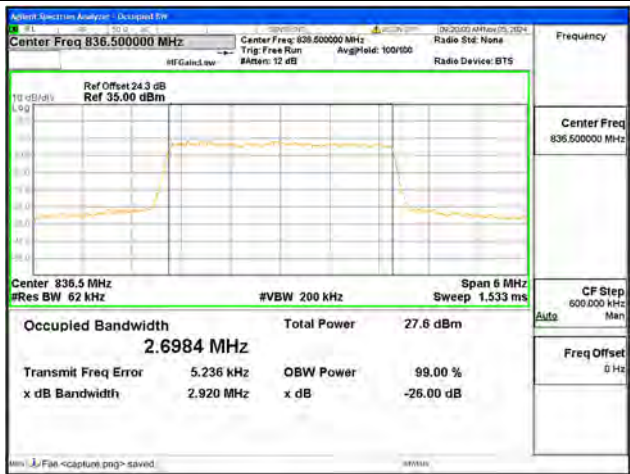
B5 / 3MHz / 64QAM/ Mid CH
