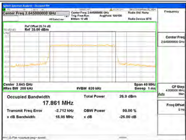
B41 / 20MHz / 16QAM/ High CH
