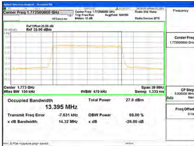
B66 / 15MHz / 64QAM/ High CH
