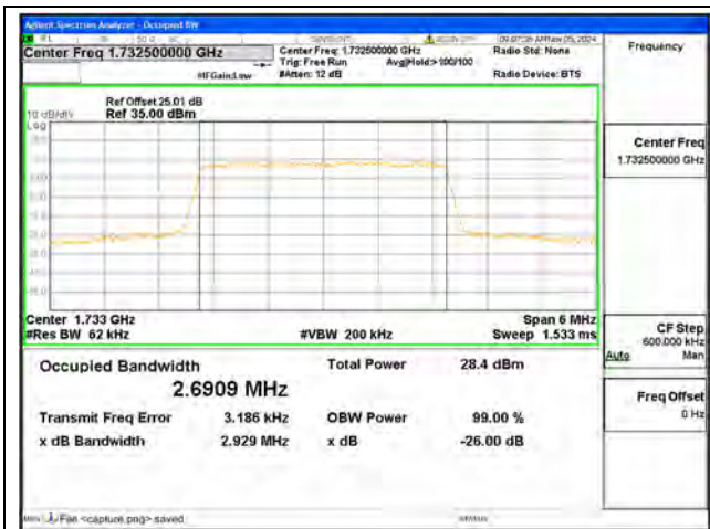
B4 / 3MHz / QPSK/ Mid CH
