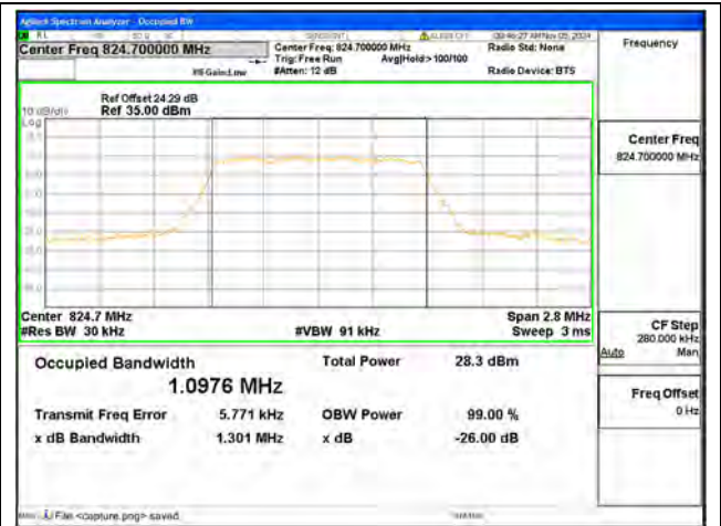
B26 / 1.4MHz / 16QAM/ Low CH
