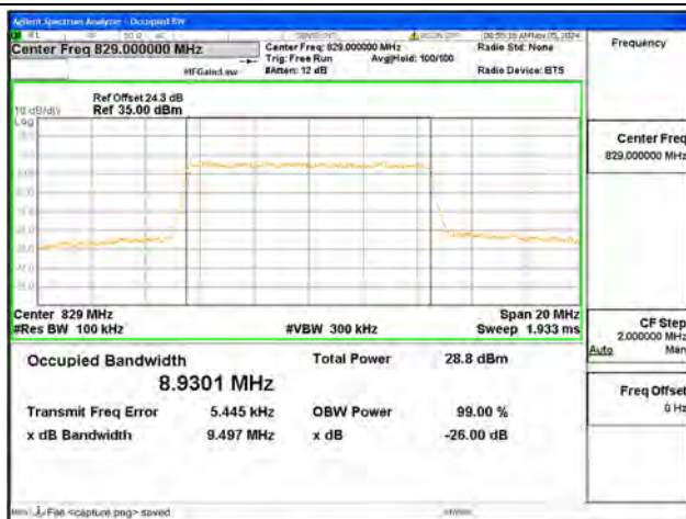
B26 / 10MHz / 16QAM/ Low CH
