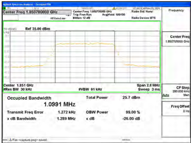
B2 / 1.4MHz / 64QAM/ Low CH
