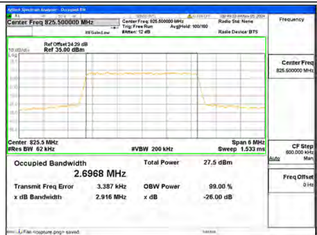
B26 / 3MHz / 64QAM/ Low CH
