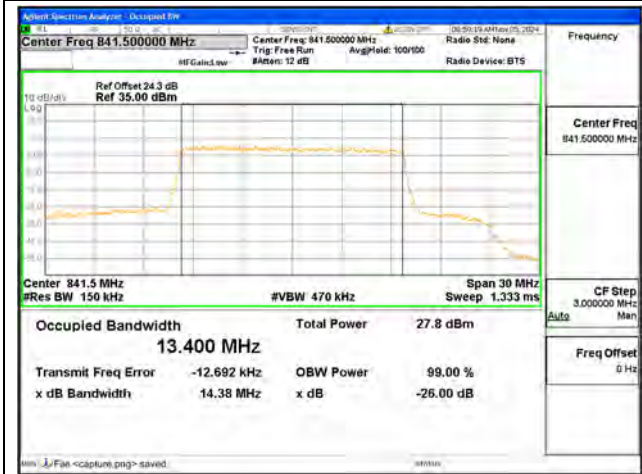
B26 / 15MHz / 64QAM/ High CH
