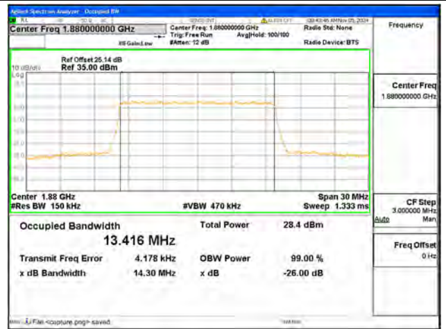
B2 / 15MHz / QPSK/ Mid CH
