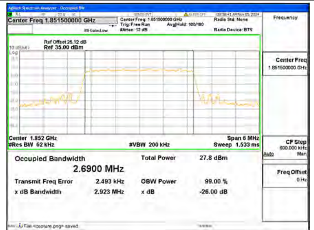
B2 / 3MHz / QPSK/ Low CH
