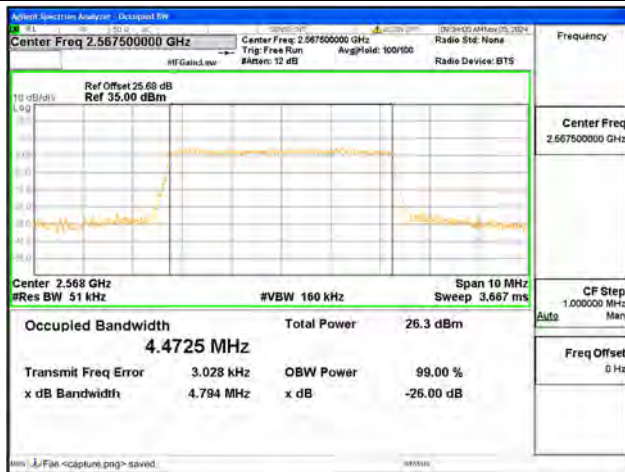
B7 / 5MHz / 64QAM/ High CH
