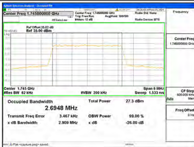
B66 / 3MHz / 64QAM/ Mid CH
