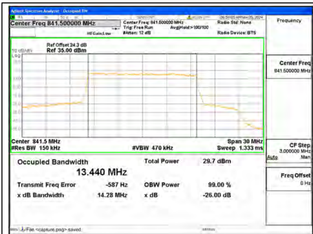
B26 / 15MHz / QPSK/ High CH
