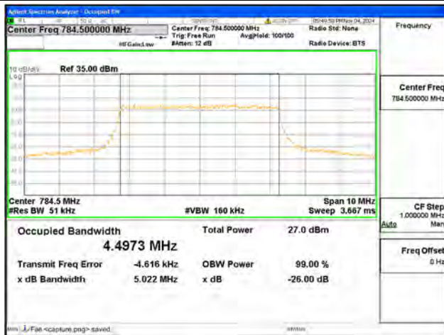
B13 / 5MHz / 64QAM/ High CH
