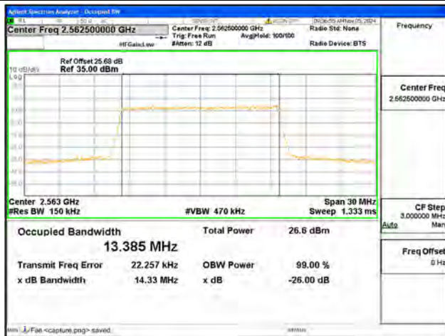
B7 / 15MHz / 64QAM/ High CH
