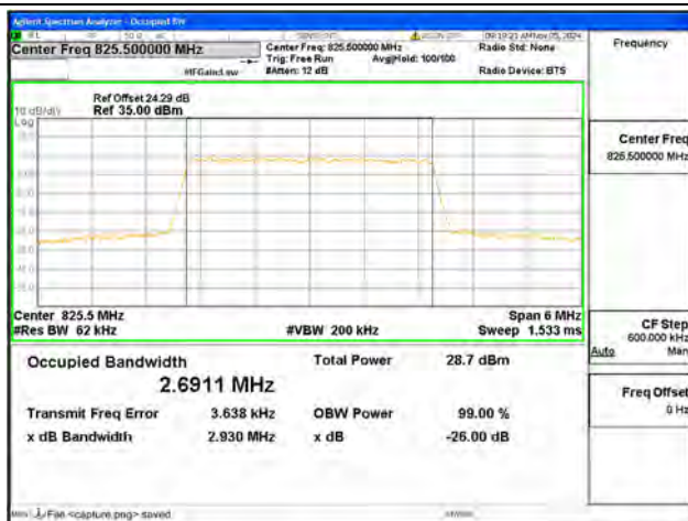
B5 / 3MHz / 16QAM/ Low CH
