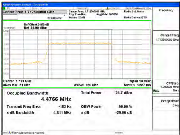
B4 / 5MHz / 64QAM/ Low CH
