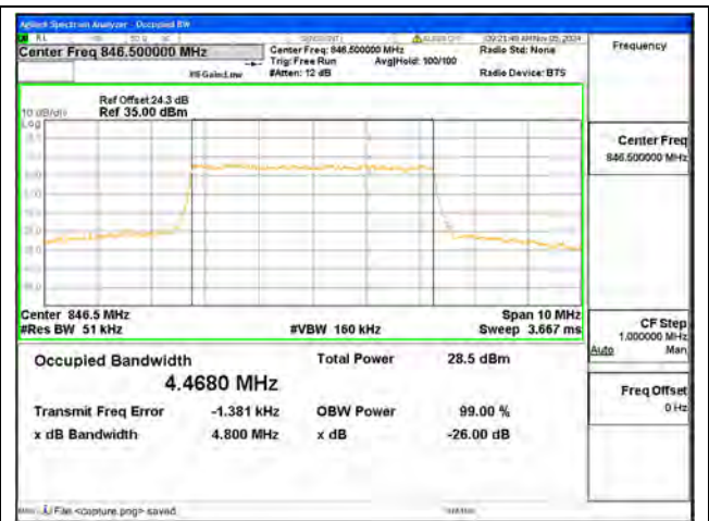
B5 / 5MHz / 16QAM/ High CH
