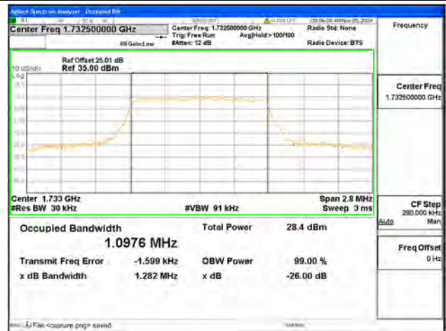
B4 / 1.4MHz / QPSK/ Mid CH
