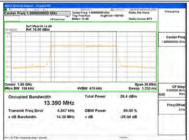
B2 / 15MHz / 64QAM/ Mid CH
