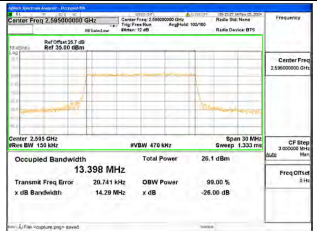
B41 / 15MHz / 64QAM/ Mid CH
