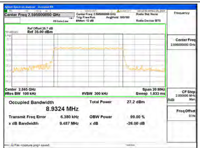
B41 / 10MHz / 16QAM/ Mid CH
