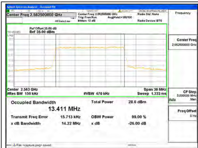
B7 / 15MHz / QPSK/ High CH
