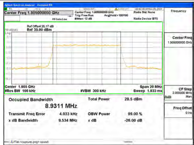
B2 / 10MHz / QPSK/ High CH
