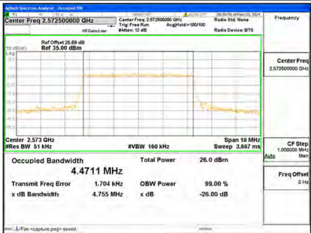
B38 / 5MHz / 64QAM/ Low CH
