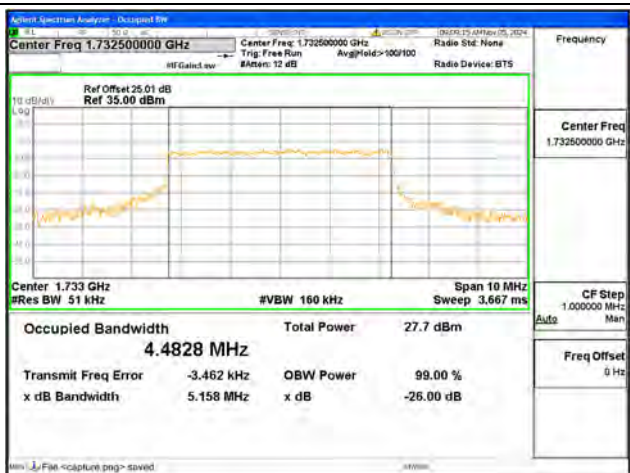
B4 / 5MHz / 16QAM/ Mid CH
