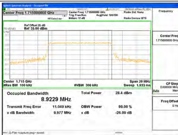
B66 / 10MHz / 16QAM/ Low CH
