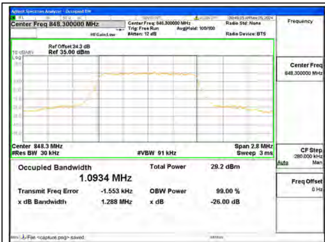
B26 / 1.4MHz / QPSK/ High CH
