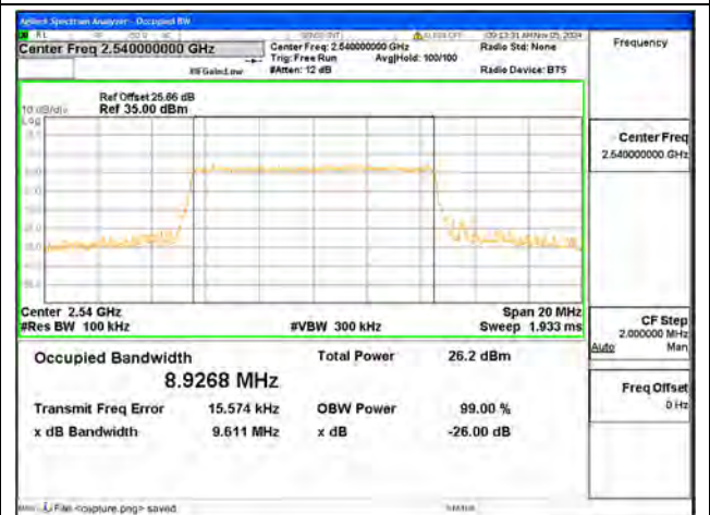
B41 / 10MHz / 64QAM/ Low CH
