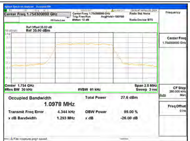
B4 / 1.4MHz / 16QAM/ High CH
