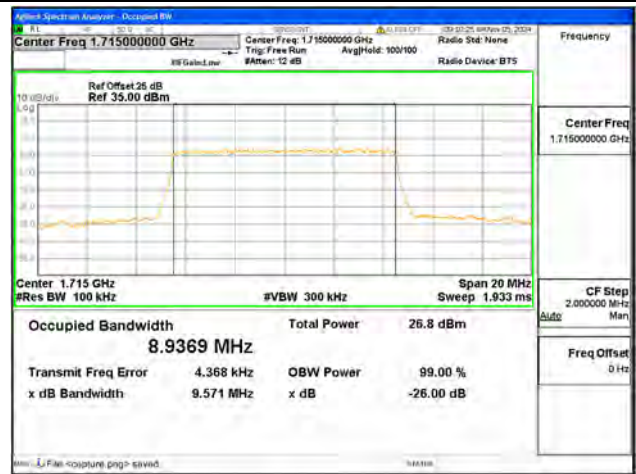
B4 / 10MHz / 64QAM/ Low CH
