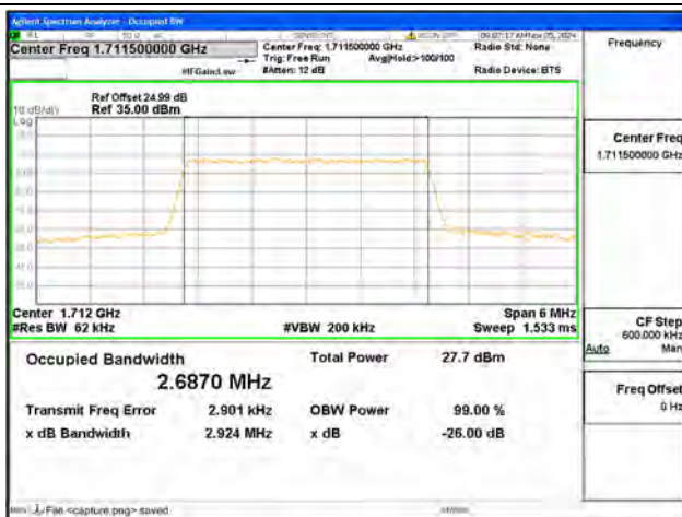
B4 / 3MHz / 16QAM/ Low CH
