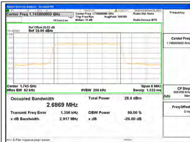
B66 / 3MHz / QPSK/ Mid CH
