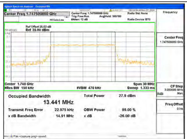
B4 / 15MHz / 16QAM / High CH
