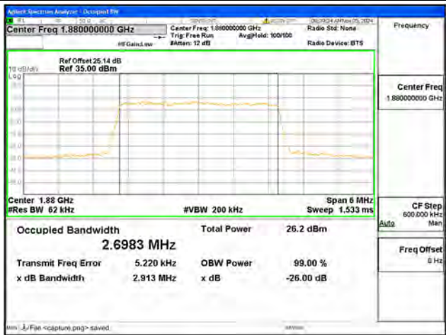
B2 / 3MHz / 64QAM/ Mid CH
