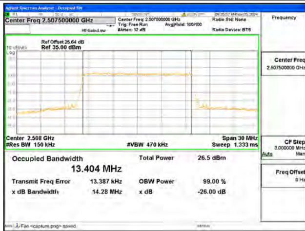
B7 / 15MHz / 64QAM/ Low CH
