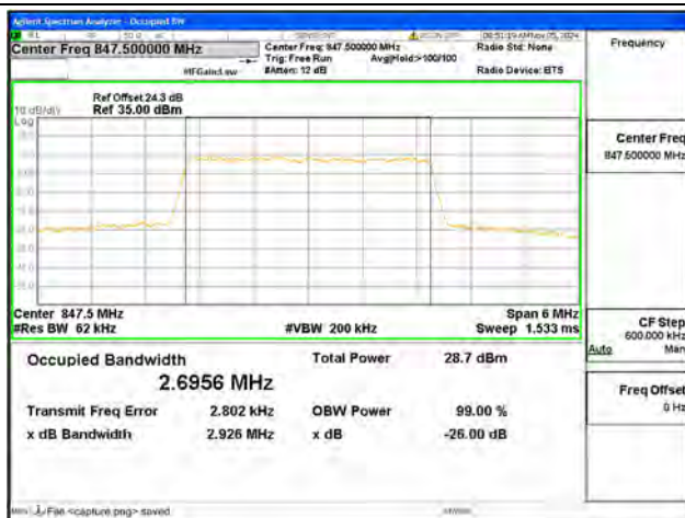
B26 / 3MHz / 16QAM/ High CH
