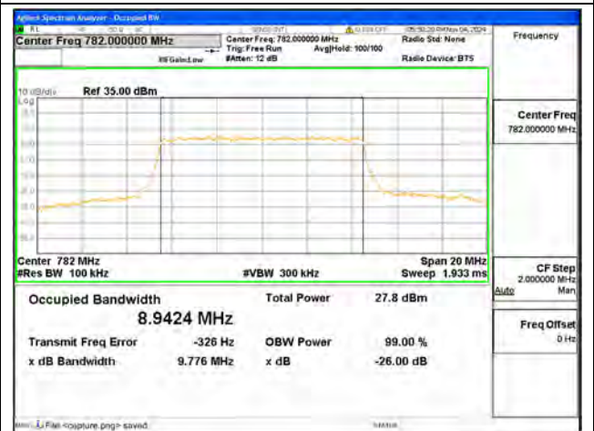
B13 / 10MHz / 64QAM/ Mid CH
