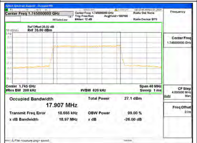
B4 / 20MHz / 64QAM/ High CH
