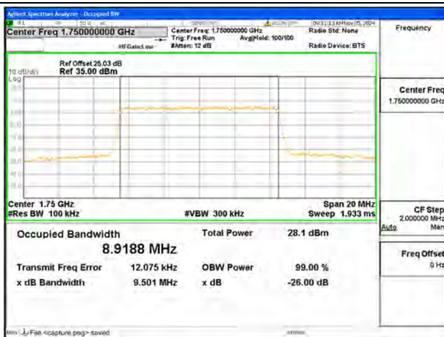
B4 / 10MHz / 16QAM/ High CH
