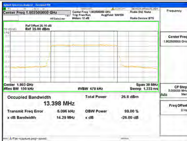
B2 / 15MHz / 64QAM/ High CH
