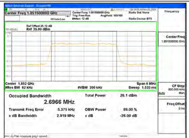
B2 / 3MHz / 64QAM/ Low CH
