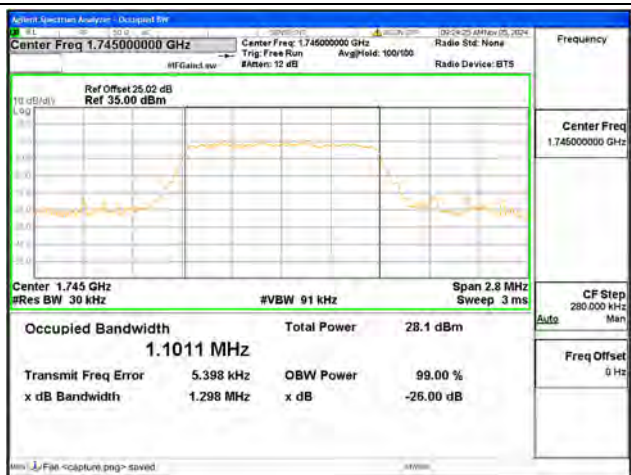
B66 / 1.4MHz / 16QAM/ Mid CH
