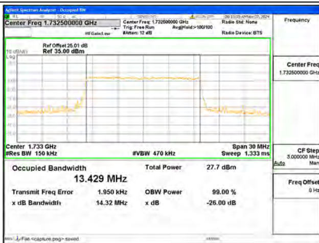
B4 / 15MHz / 16QAM/ Mid CH
