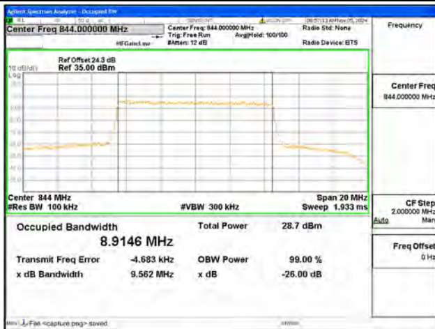
B26 / 10MHz / 16QAM/ High CH
