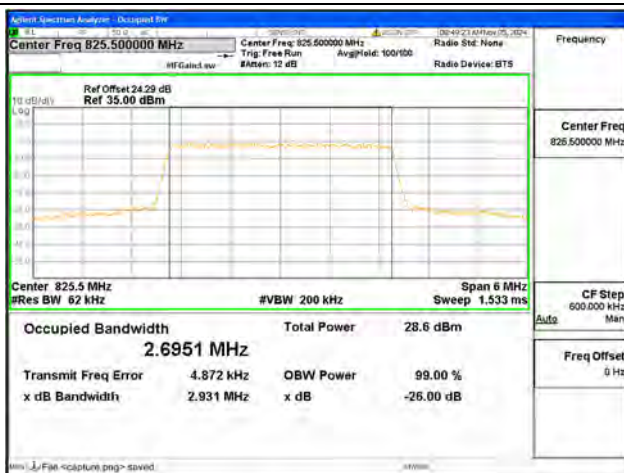
B26 / 3MHz / 16QAM/ Low CH
