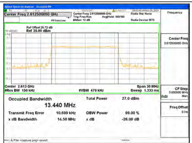
B38 / 15MHz / 16QAM/ High CH
