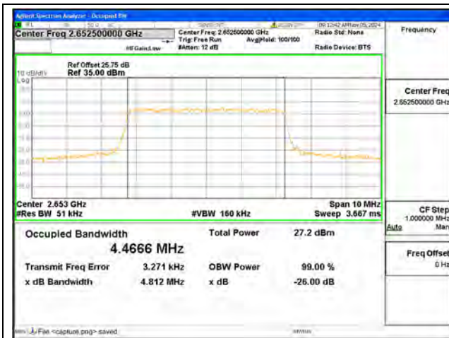
B41 / 5MHz / QPSK/ High CH
