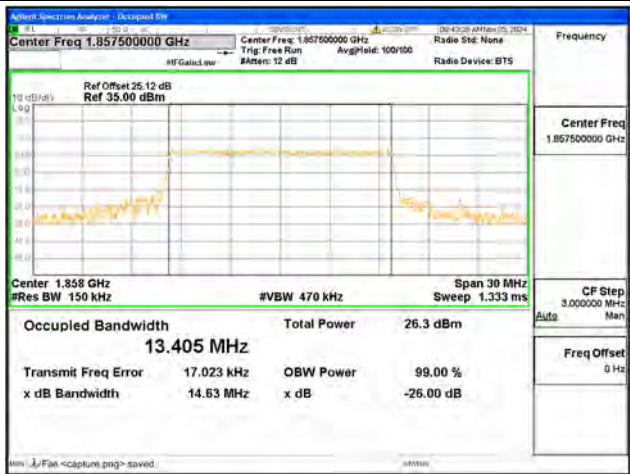
B2 / 15MHz / 64QAM/ Low CH
