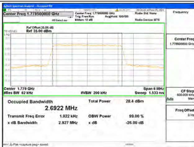
B66 / 3MHz / 16QAM/ High CH
