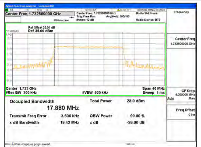
B4 / 20MHz / 16QAM/ Mid CH
