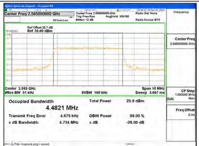
B38 / 5MHz / 64QAM/ Mid CH
