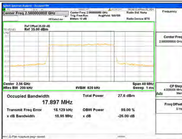
B7 / 20MHz / 16QAM/ High CH
