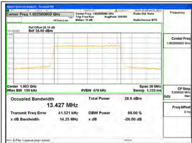
B2 / 15MHz / QPSK/ High CH
