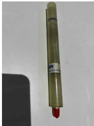
Fig 2 dipole model 3126-2500 frequency 2500 MHz
