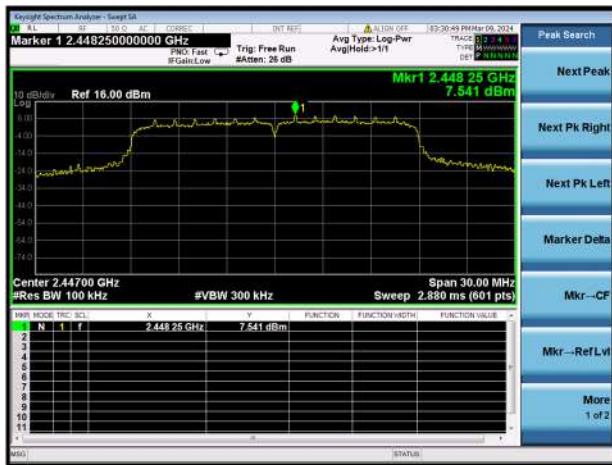
802.11n-20 MHz CH8, CARRIER LEVEL
