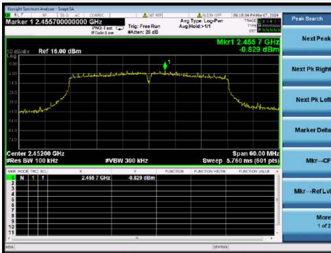
802.11n-40 MHz CHANNEL 9, CARRIER LEVEL
