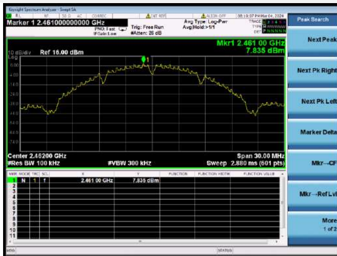
802.11b CHANNEL 11, CARRIER LEVEL
