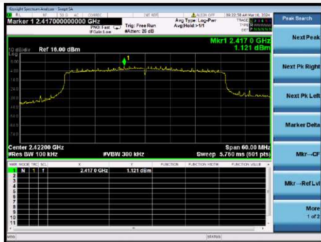
802.11ax-40 MHz(SU) CHANNEL 3, CARRIER LEVEL
