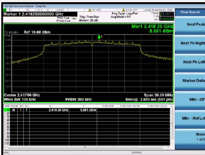
VHT-20 MHz CHANNEL 2, CARRIER LEVEL
