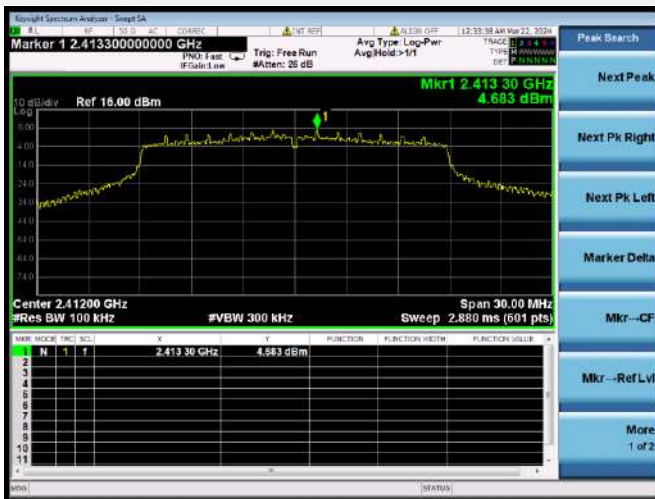
VHT-20 MHz CHANNEL 1, CARRIER LEVEL
