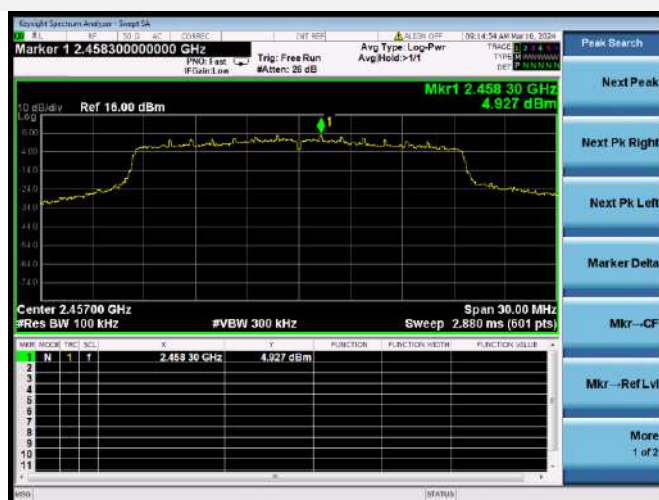
802.11ax-20 MHz(SU) CHANNEL 10, CARRIER LEVEL
