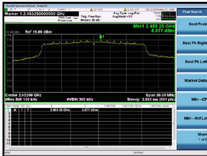
802.11ax-20 MHz(SU) CHANNEL 9, CARRIER LEVEL
