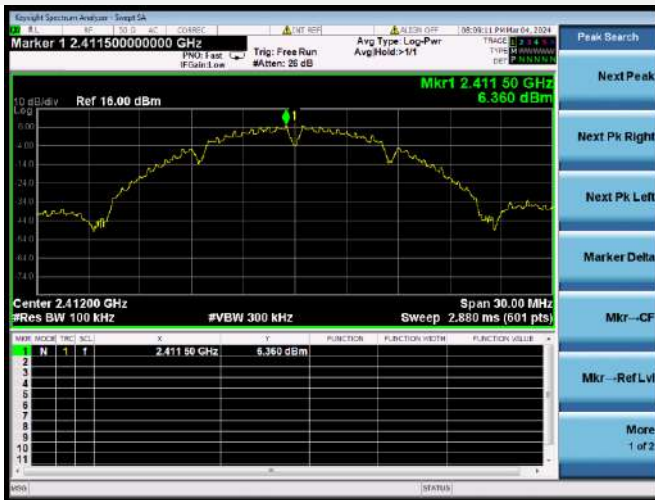
802.11b CHANNEL 1, CARRIER LEVEL
