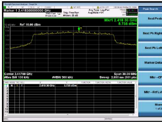
802.11ax-20 MHz(SU) CHANNEL 2, CARRIER LEVEL
