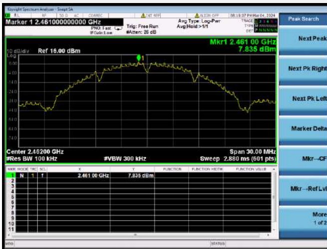
802.11b CHANNEL 11, CARRIER LEVEL
